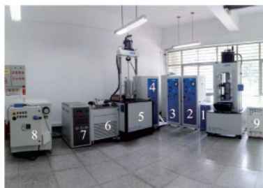
图1 FRTR-1500高/低温高压差岩土静/动力学测试系统 Fig.1 FRTR-1500 high/low temperature and high pressure differential geostatic/dynamic testing system
